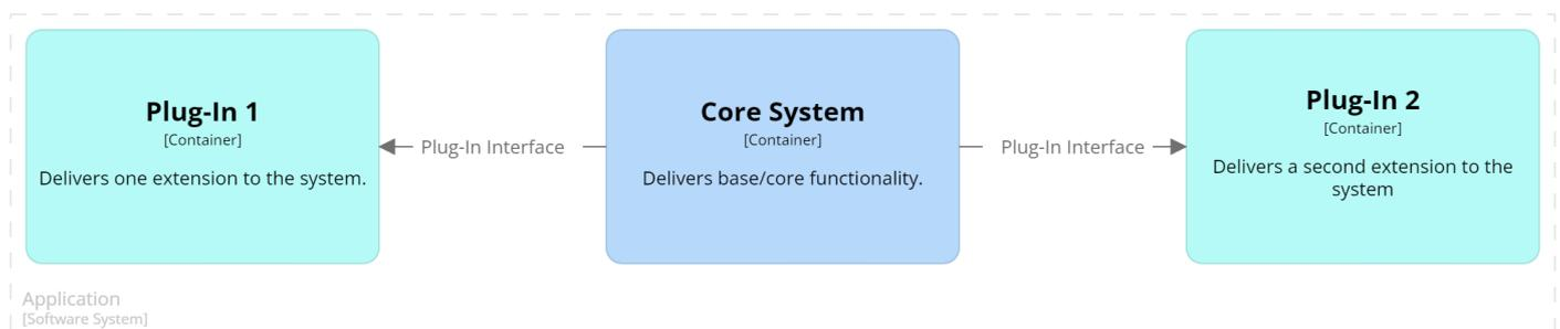
Figure 1: Generic structure of the microkernel architecture.
