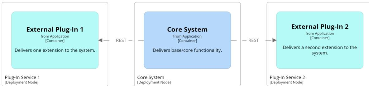
Figure 7: Microkernel architecture – separate plug-in services using REST.
