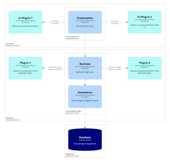
Figure 6: Microkernel architecture distributed by technical partitions.
