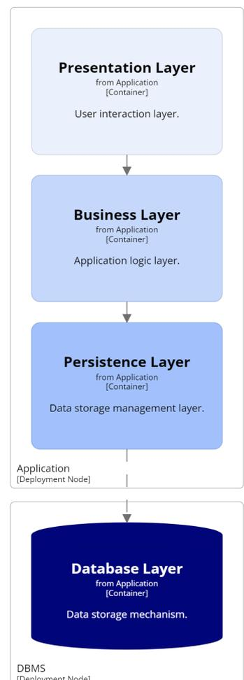
Figure 3: Layered architecture as example of technical partitioning.
