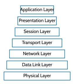
The above diagram shows the layers of the *OSI* model. These are the layers of abstraction that comprise the Internet Protocol Suite (or, how computers communicate over the Internet).
