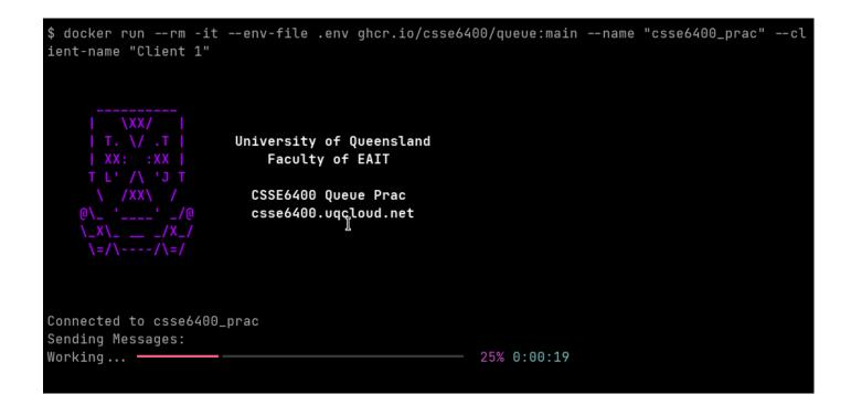
When the publisher connects to the queue it is going to put 100 messages of increasing increment into the queue. On the subscriber we will be able to see the messages being received, an example is provided below:
